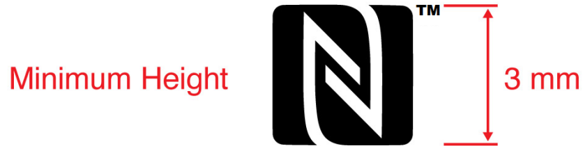
Figure 4: Minimum Height Requirements
